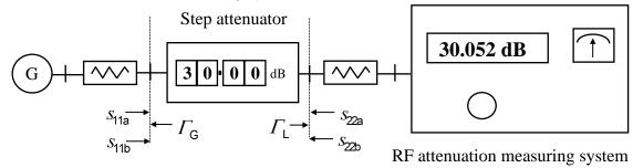
**S7.3** The attenuation  $L_x$  of the attenuator to be calibrated is obtained from the relation:
